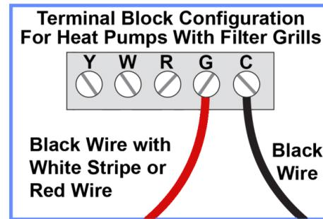
For a heat pump with filter grill(s) connect the black wire with white stripe (or red wire) to G and the other wire to C. Doing so will energize the air cleaner only when the fan operates. See diagram (Terminal Block Configuration for Heat Pumps With Filter Grills)
